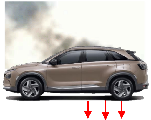
Hydrogen Gas Venting Direction
