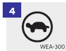
4 : Power Down Warning Light indicates that there may be a malfunction with the fuel cell stack. When it comes on during driving, the vehicle power will be limited.
